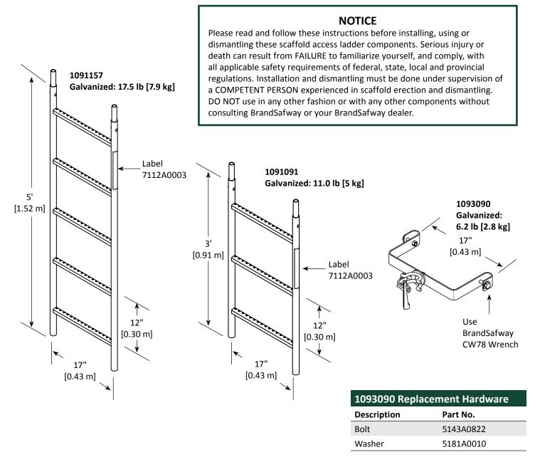
Use these installation instructions for 1091157, 1091091 and 1093090 when used with SafLock frame and brace, and tube and clamp scaffolds.
