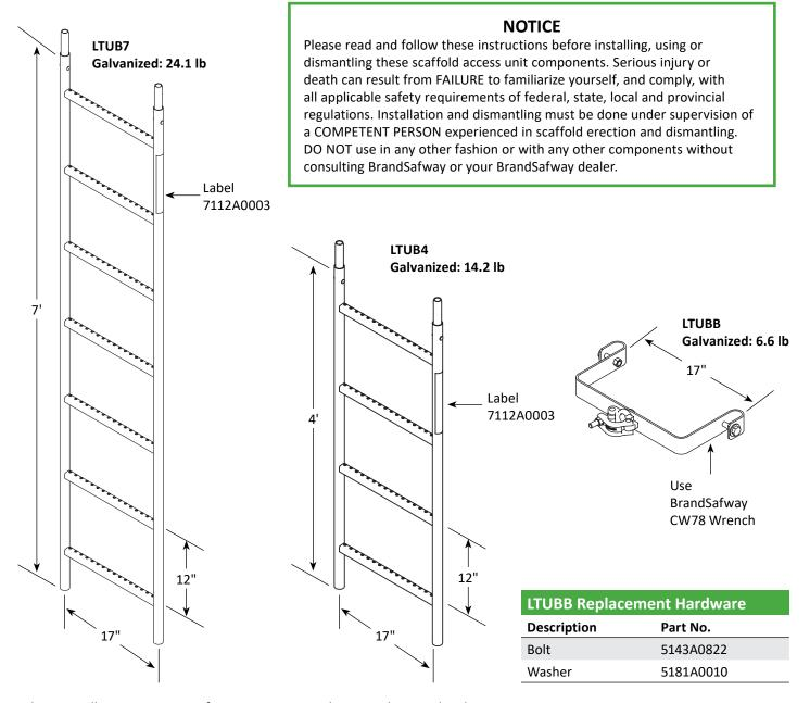
Use these installation instructions for LTUB7, LTUB4 and LTUBB when used with BrandSafway Systems™, Sectional and Tube and Clamp scaffolds.
