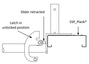
\* Ensure SSP\_Plank and Horizontals will support all applied loads, including point loads from one (1) 250 worker, including tools.
