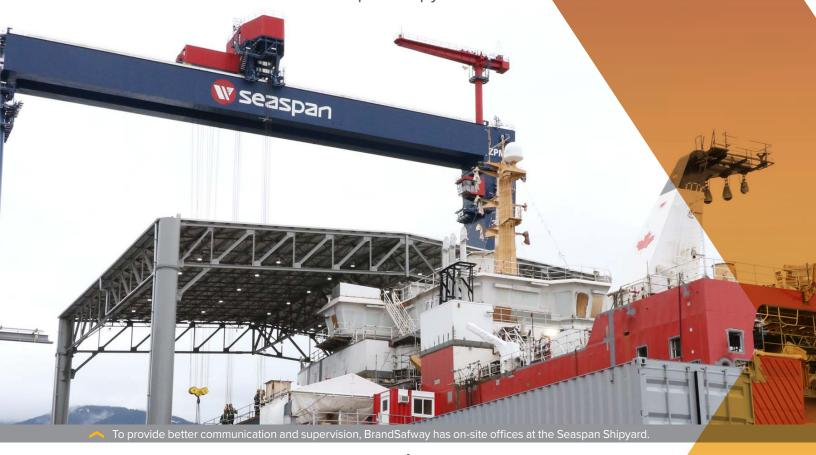
Modern ship construction resembles a giant Lego project, with a bit of jigsaw puzzle and Rubik's Cube thrown in for good measure. Instead of laying a keel and building the vessel as a whole, shipyards fabricate individual blocks, assemble the blocks into grand blocks, join the grand blocks into bow-, mid- and stern-rings, and then finally connect all the sections to create a ship.
